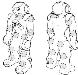
Figure 3: Keep fingers out of the joints!
